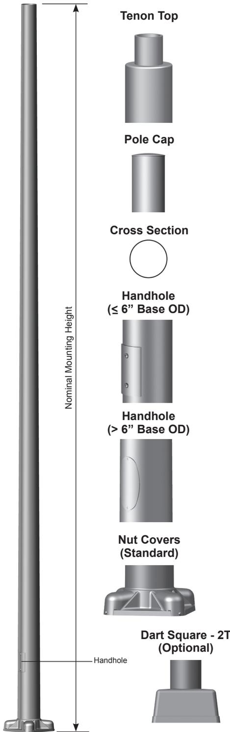
**Pole** - The pole shaft is spun from seamless alloy aluminum.
